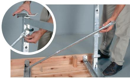
The Leg Frame Brace fits into a slot on the underside of the dock and is secured to the dock leg pin with a hairpin cotter key.
