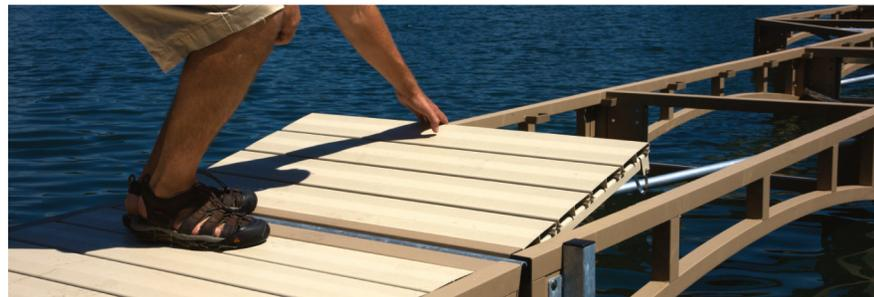
Once the frame sections are positioned, it's time to add the deck. The lightweight, easy-to-handle 2'x4' drop-in deck sections lock into place with spring snaps, no tools needed.
