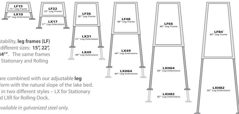
For maximum adjustability, **leg frames (LF)** are available in six different sizes: **15", 22", 36", 48", 66"** and **84"**. The same frames are used with both Stationary and Rolling Dock systems.
